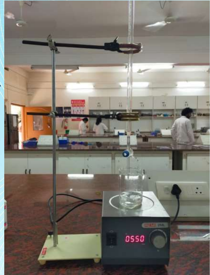
Ethanol is added to zinc acetate+NaOH mixture
